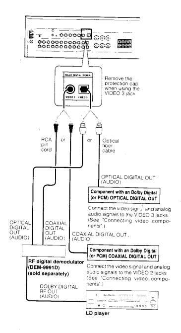
To connect an LD player with a DIGITAL RF OUT, connect the LD player to the KENWOOD RF digital demodulator (DEM-9991D)
